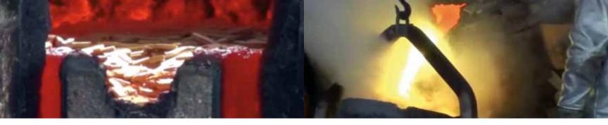
Above left: keys melting in crucible at Bollinger Atelier, Tempe, Arizona. Above right: molten brass being poured into sand cast molds.
